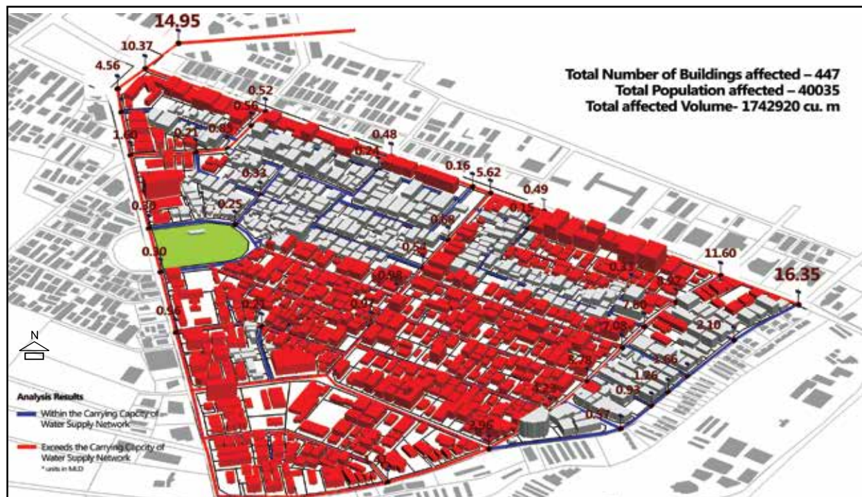
Fig. 11: Water Supply Networks Analysis Result of the Study Area and Critical Network 2013
